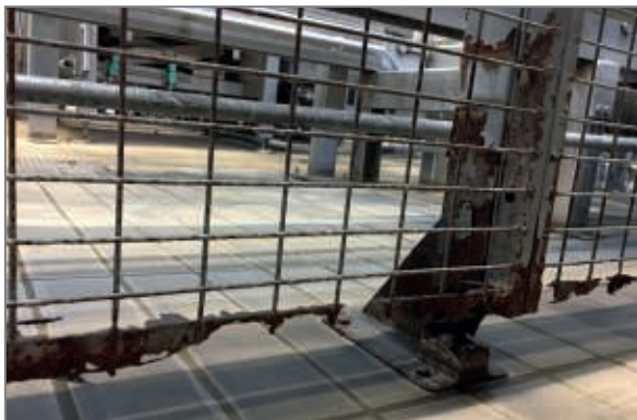
In the food processing industry, guarding solutions in corroded conditions like this, are unfortunately still seen.
