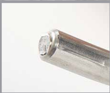
7) V-chamfering CNC. Mechanical. Smooth outside. Burr inside.
