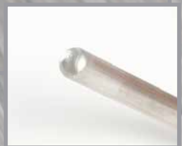
6) Soft end – melted.
