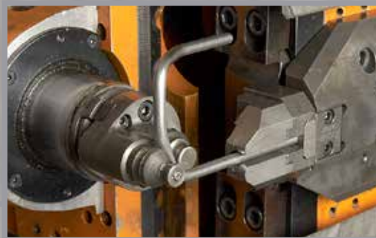
8) V-groove CNC. Mechanical. For locking ring, embedment or similar.
