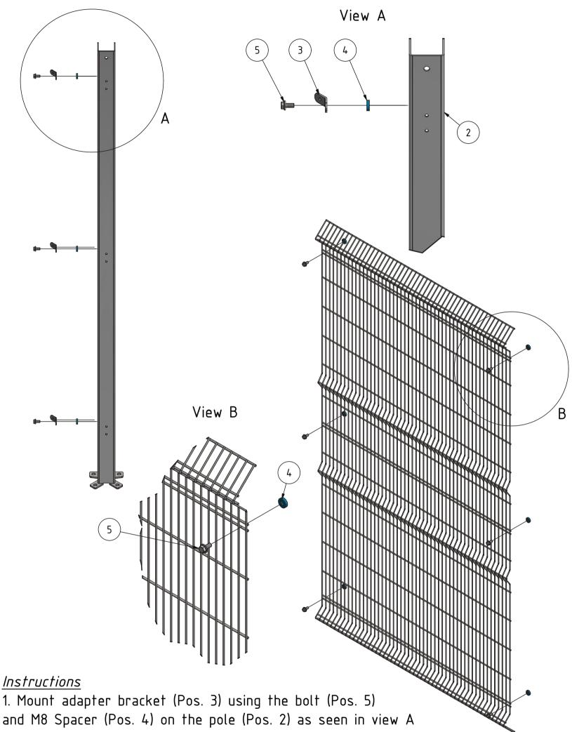
and M8 Spacer (Pos. 4) on the pole (Pos. 2) as seen in view A
